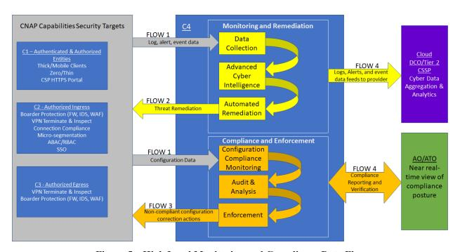
Figure 5 - High Level Monitoring and Compliance Data Flow
